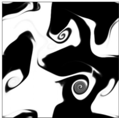
Figure 9. Two-dimensional simulation of the mixing of two educt flows under turbulent conditions. [77]
